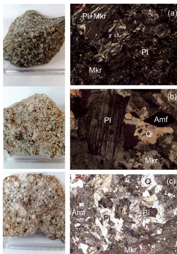
Figure 4. Photomacrographs and photomicrographs (cross-polarized light) for rocks of the Uskalin massif. (a) granosyenite (Sample d2010–3); (b) subalkaline granite (Sample d2010–1); (c) quartz diorite porphyrite (Sample d2010–2). Q – quartz, Pl – plagioclase, Amp – amphibole, Bi – biotite, Mkr – K-Feldspar.
