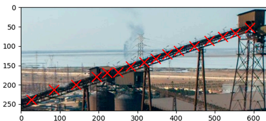
Figure 5. Tiltrotor quadcopter path of 74 meters along the transition tower and conveyor. The red targets indicate the tiltrotor path.
