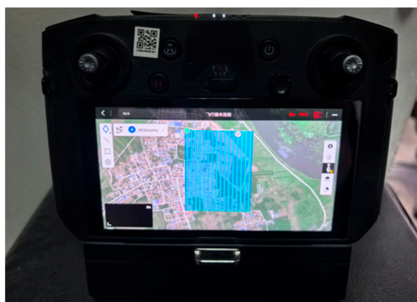
Figure 5. DJI UAV remote controller and flight route planning.
