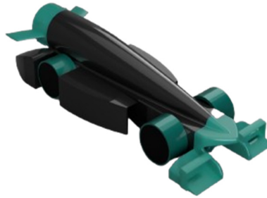
Figure 13(a) Isometric View of the Final Brian Variant Statistics- Total Area: 632.67 cm 2 Drag Force: 2.17N Drag Coefficient: 0.22
