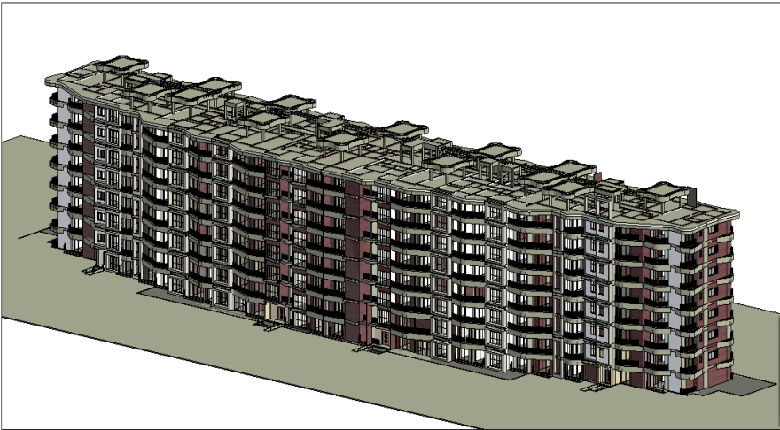
Figure 31. 3D Architectural BIM model of the project (LOD 300)
