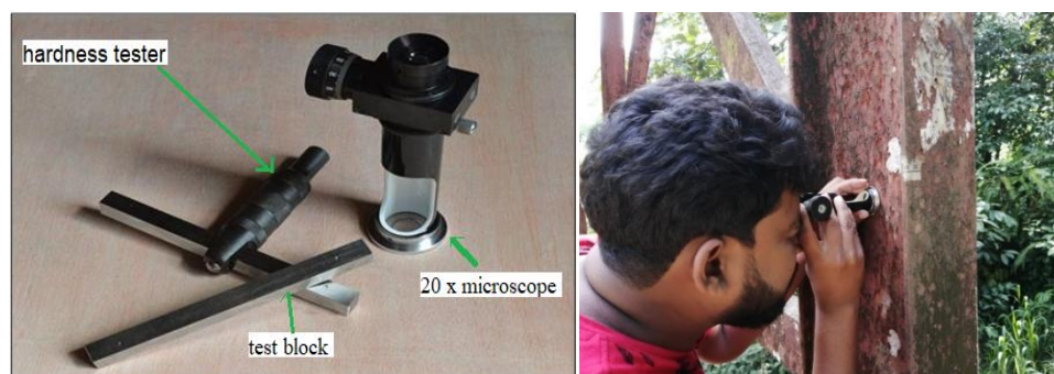
Figure 1. Brinell hardness Tester and its use.
