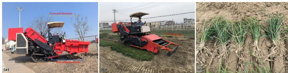
Figure 13. Field trial validation and operational performance demonstration: (a) Prototype root–soil separation device and soil collection zone schematic; (b) Field operation process and forward direction; (c) Separated Ophiopogon japonicus plant samples (used for soil retention and separation efficiency evaluation).
