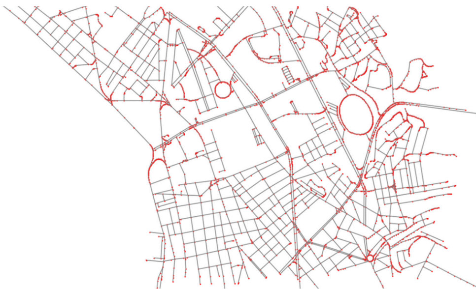
Figure 5. Example of a graph of the street network of a part of Thessaloniki's center where nodes represent intersections, and edges signify road segments.
