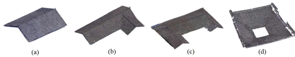
Figure 9. Extraction results for building roofs:(a)I-shaped; (b)L-shaped; (c)U-shaped; (d)回-shaped.
