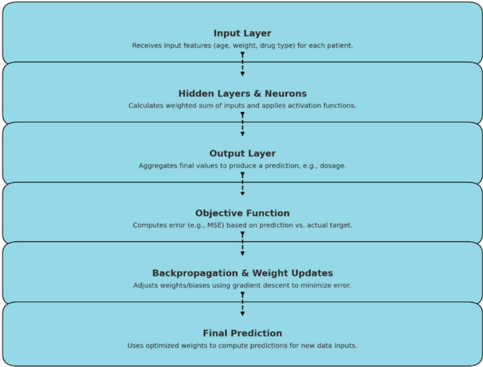
Figure 3. 0: flow chart illustrating the AnaMo model’s output computation process.
