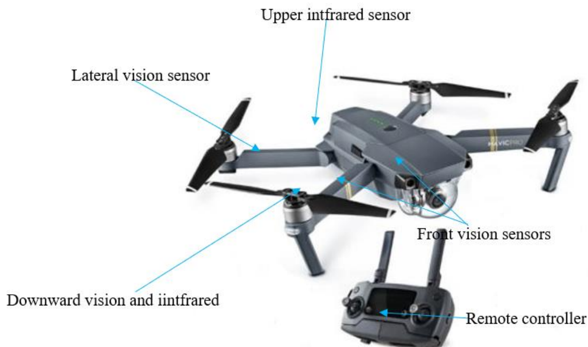
Figure 3. DJI Mavic 2 Pro and its components (source: Dronezon.com).
