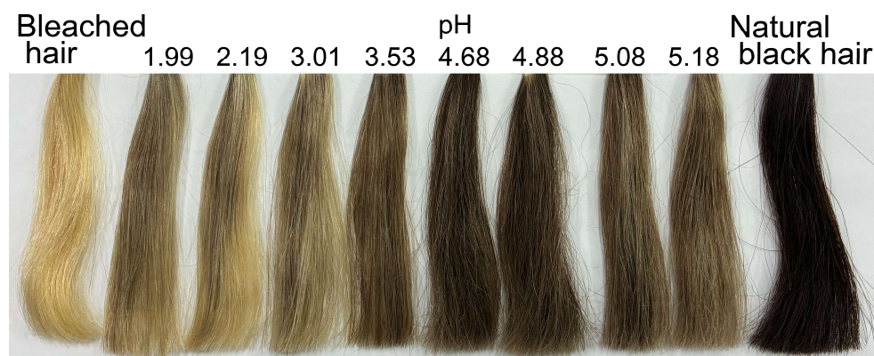
Figure 6. Photographs of bleached hair tresses treated with the SIP–chitosan system at a fixed SIP:chitosan weight ratio of 10:1 at different pH values.
