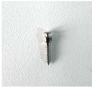
Figure 1. 1.8 x 0.8 mm miniscrew used in the study.
