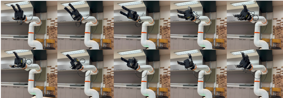
Figure 3. 10 sampling poses used for calibration throughout this paper. These postures are selected by rotating the wrist angle in the orientation that generates the highest torque, allowing for various orientations.
