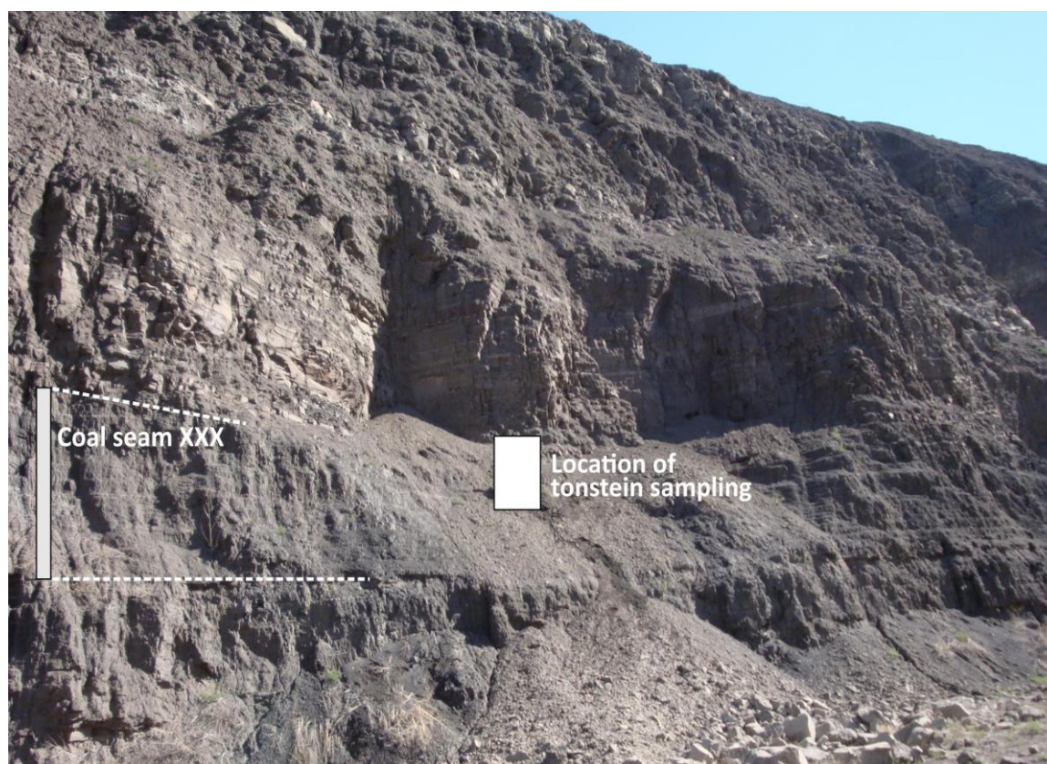
Figure 6. Outcrop of the upper part of the Izykh Fm in the Izykh coal mine showing the location of tonstein sampling.
