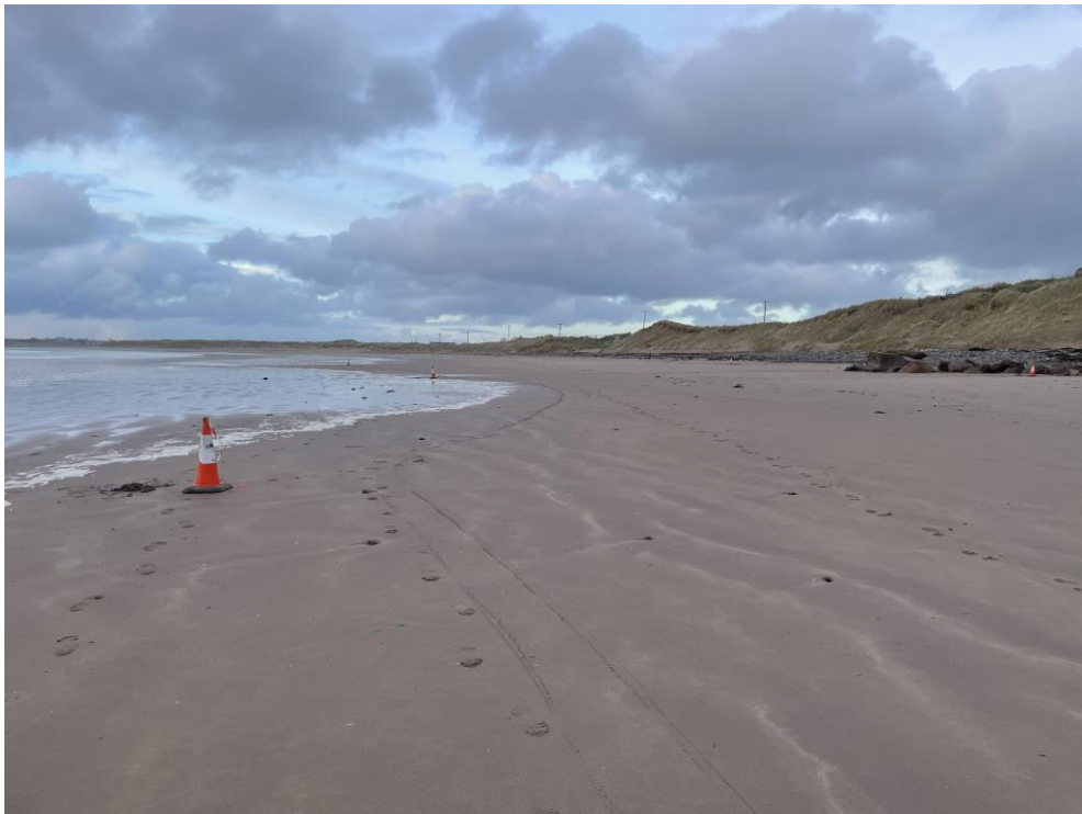
Figure 5. Road traffic cones were placed in the field and used as temporary GCPs.
