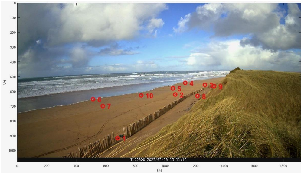
Figure 6. Temporary GCPs used in the field (Camera 2).
