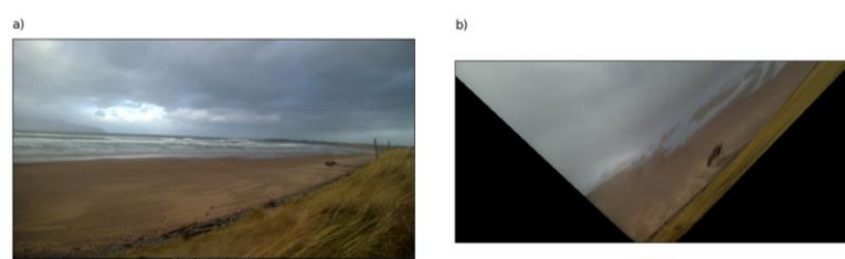
Figure 12. Example of a) snapshot, and b) resulting Timex image during receding tides, showing remaining water on the beachface resulting in shoreline edge detection not representing the actual shoreline (from 26 February 2022 at 10h).
