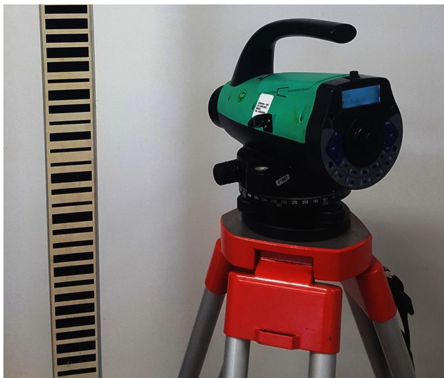
Figure 4. Example of a digital level – bar-code staff system.
