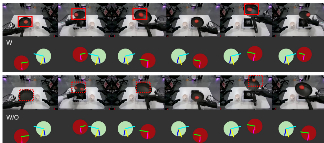
Figure A1. Results of generated videos under identical conditions with and without the Delta Action Module. The top row shows results with the module (w/ Delta Attention), while the bottom row shows results without it (w/o Delta Attention). The dashed red boxes highlight regions with inconsistent or hallucinated results.
