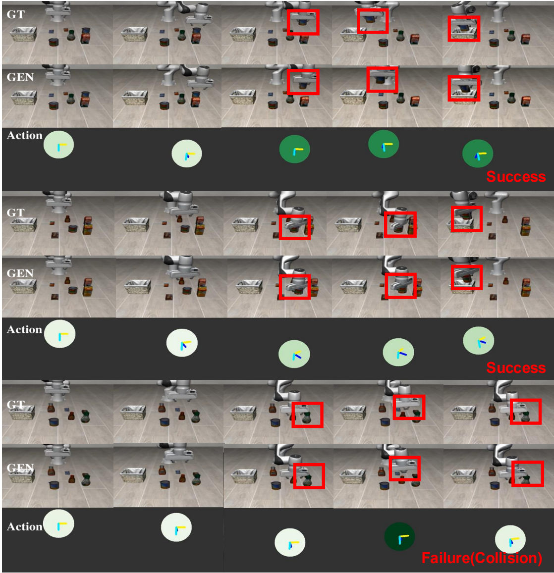
Figure A3. Comparison of results generated by Libero and EVAC with different action trajectories. Two successful cases of picking an item are shown, along with one failure case of an empty catch.
