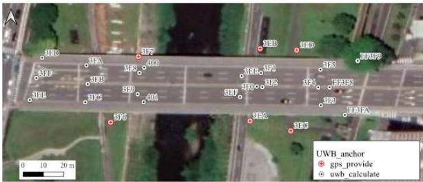
Figure 12. The 166-meter-long bridge is deployed with a total of 27 UWB anchors along its span.
