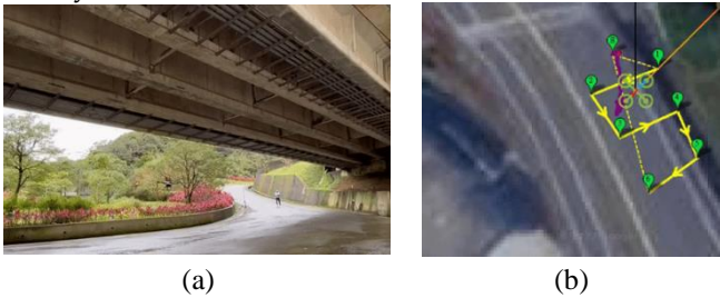
Figure 13. (a) Drone's flight trajectory (b) Pre-defining path via Mission Planner. The purple line represents the actual flight path of the drone.
