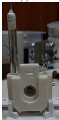
Figure 3. electrochemical cell for Raman spectroscopy in situ, described in Santos [87].
