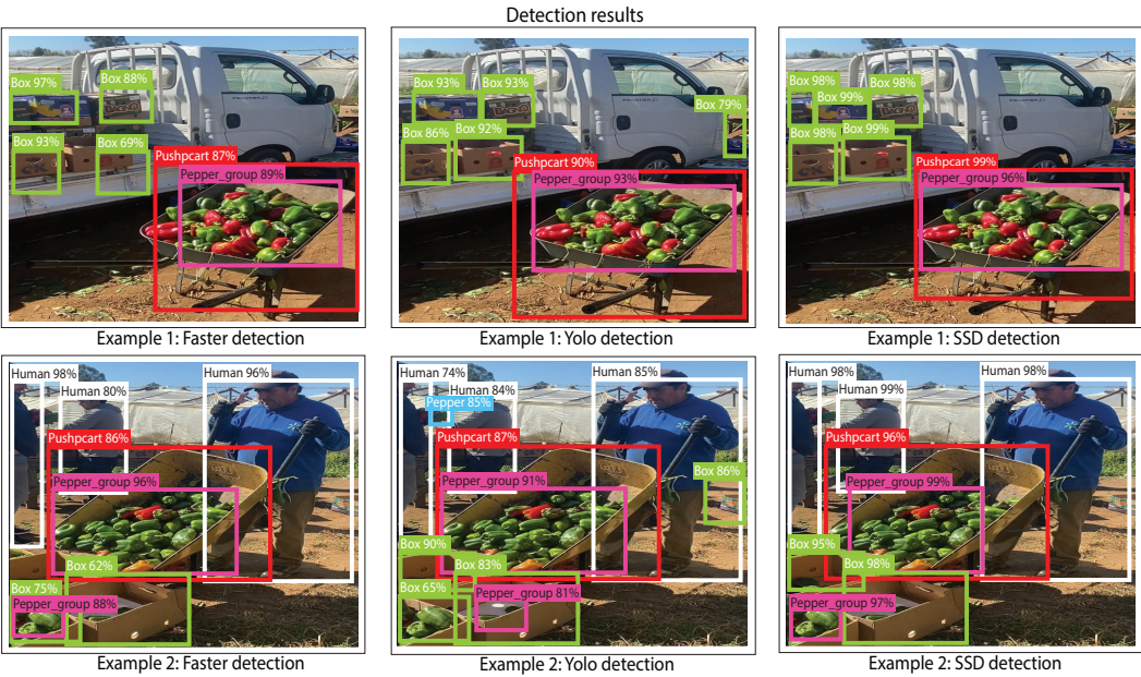
Figure 15. Object detection during Pepper harvesting processes with ShuffleNet as a feature extractor for Faster R-CNN, YOLOv7, and SSD.
