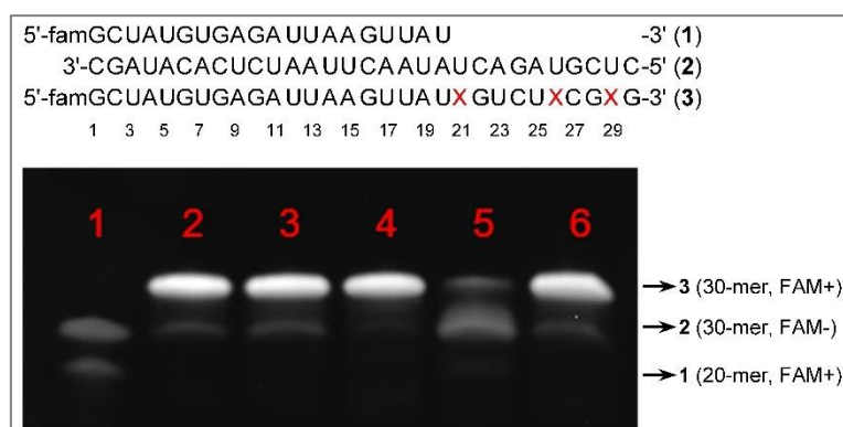
Figure 1. Image of denatured PAGE for the analysis of SARS-CoV-2 RdRp catalyzed RNA polymerization reactions. X in 3 is the nucleoside A or m 1 A depending on the NTP used. The mixture of RdRp, primer-template duplex 1-2 and NTPs was incubated at 37 °C for 2 h. The reaction products were analyzed with PAGE. The image was taken after staining with GelRed. Lane 1: RNA duplex only. Lane 2: ATP, CTP, GTP and UTP, no m 1 ATP. Lane 3: m 1 ATP, CTP, GTP and UTP, no ATP. Result indicates that m 1 A can be incorporated into RNA via m 1 ATP. Lane 4: m 1 ATP only for 15 min, then ATP, CTP, GTP and UTP. Results indicate m 1 ATP does not inhibit RdRp. Lane 5: CTP, GTP, UTP, no ATP, no m 1 ATP. Results indicate that ATP and m 1 ATP in other lanes were needed.
