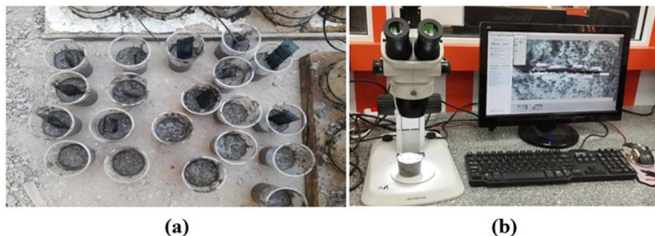
Figure 7. (a): Creation of visible cracks, and (b): The experimental device for measuring visible cracks.
