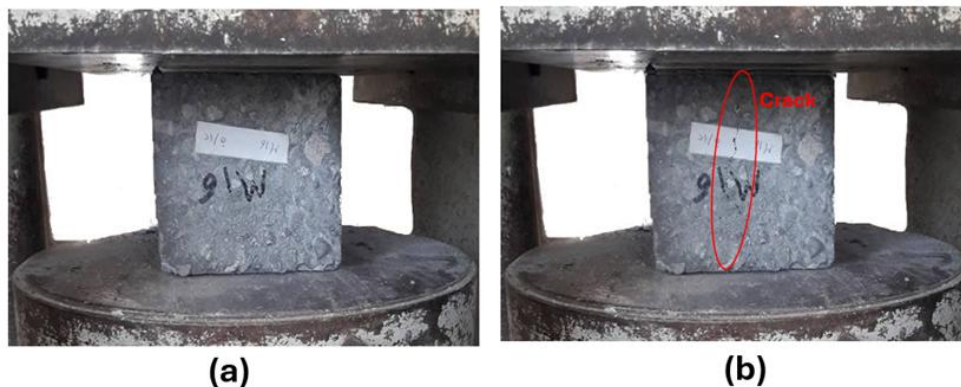
Figure 6. (a) Specimen before cracking. (b) Specimen after cracking.
