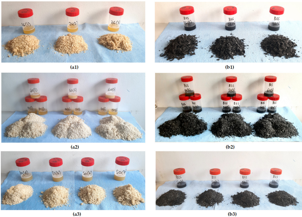
Figure 3. Extracted crude oil with sediments following the factorial design for yellowish sesame (a1 – a3) and blackish sesame (b1 – b3) for the control temperature of 24 °C (a1 and b1) and heating temperatures of 40 °C, 50 °C and 60 °C (a2, a3, b2 and b3) for various heating times of 15, 30 and 45 min.
