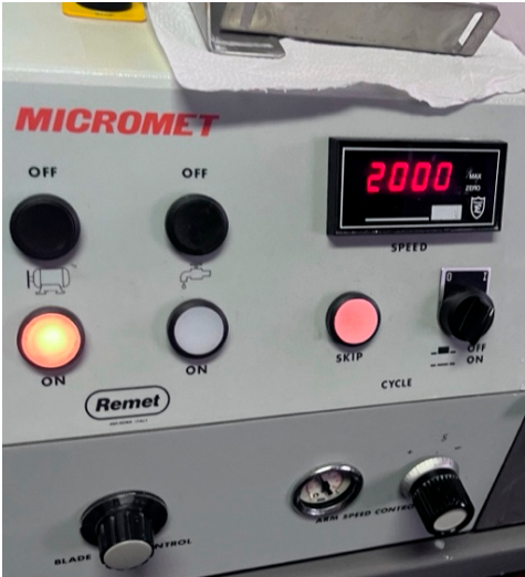
3a: 320-µm cutting machine settings (Remet s.a.s. Bologna, Italy).
