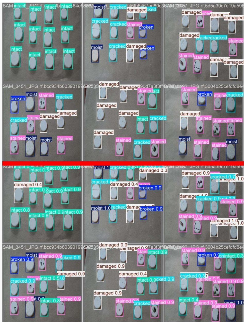
Figure 13. Qualitative comparison between ground-truth annotations (top) and YOLO11l predictions (bottom) on representative effervescent tablet test images. Each tablet is enclosed in a coloured bounding box with its class label; predicted boxes additionally show the model's confidence score.
