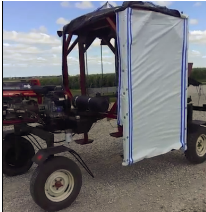
Figure 4. MARS moving out to capture soybean images
