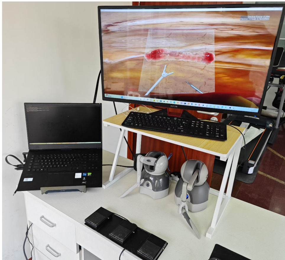
Figure 1. Hardware configuration of the proposed virtual surgical simulation platform. The interface consists of two haptic devices, foot pedals for electrocautery activation, and a high-resolution display for surgical scene visualization.
