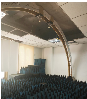
Figure 3. Arch-based reflection loss test system.
