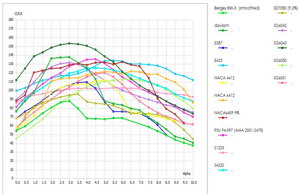
Figure 1. CL/CD vs AOA of high-performance low Reynolds number airfoils ( Re=6 \times 10^5 ).
