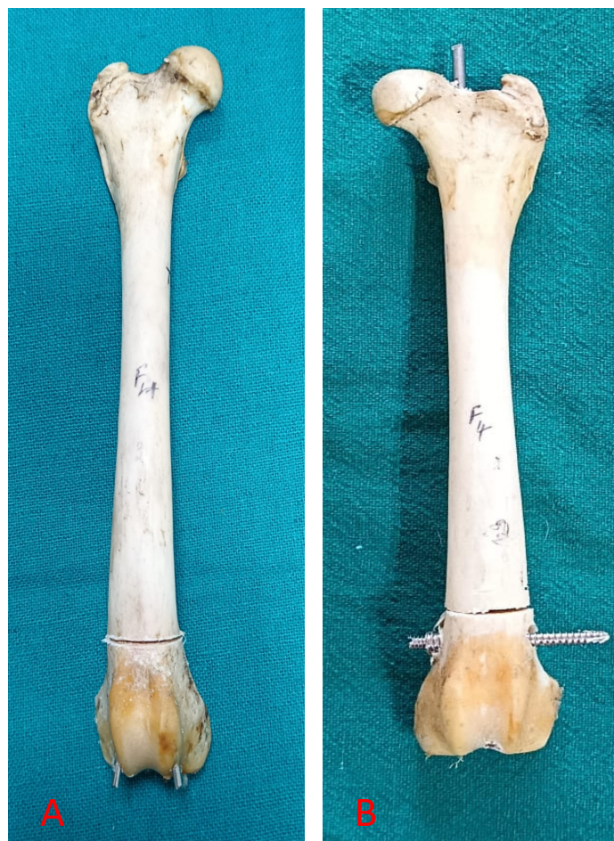
Figure 2. Constructs prepared for biomechanical testing. (A) Dynamic cross pinning configuration. (B) Locking screw–intramedullary pin construct prior to mechanical testing.
