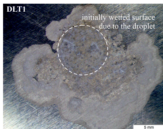
Figure 10. Photograph of corrosion site DLT1 taken at the end of the experiment. The large amount of NaCl crystals, the repeated drying and re-wetting caused deliquescence over a larger area than the initially wetted area.
