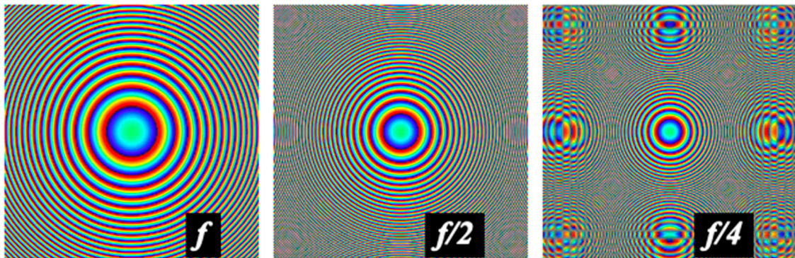
Figure 1. Modelling of SLM aliasing. The SLM has been configured to generate Fresnel lenses of different powers (1x, 2x, 4x) approaching the SLM pixel resolution. White backlight is used, and a polarizer is set so that phase delays develop colors. Aliasing becomes slightly apparent in the second lens and quite noticeable in the third lens.
