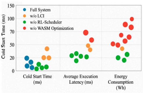
Figure 4. Performance of Each Optimization Module in the Task Scheduling System.
