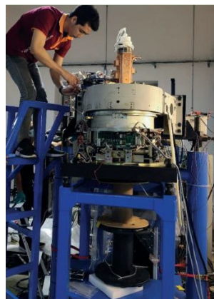
Figure 3. Linear accelerator 6 MeV for X-ray irradiation to sterilize fresh fruits by the Synchrotron Light Research Institute, Thailand.
