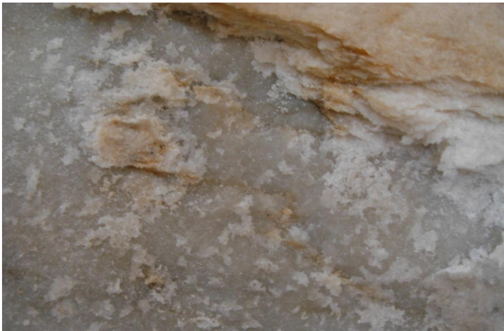
Figure 16. Multilayer exfoliation of marble. Enlargement of Figure 11.
