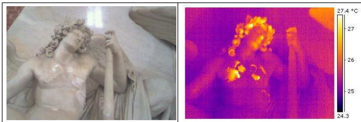
Figure 5. a) The Sleeping Genius. b) The hairs of the Sleeping Genius appear yellow at IR observation: this indicates some not visible detachments of marble surface (Courtesy of Camuffo).
