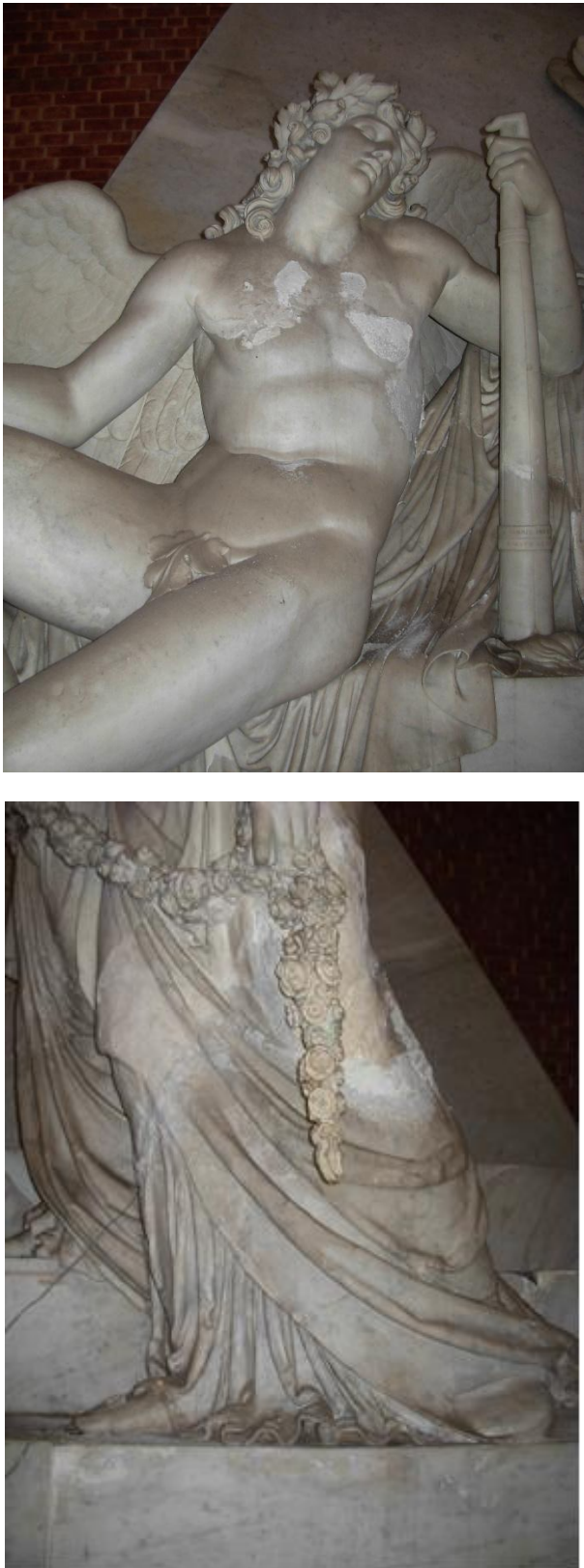
Figure 2. a) Detail of marble exfoliation on the chest of the Sleeping Genius showing the underlying whitish salt crystal. b) Detail of the marble exfoliation of the garments of Painting and Architecture .
