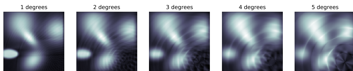
Figure 5. Reconstruction degradation: the projection interval was crucial for reconstruction. Note the image degradation going from a projection interval of 1 degree to 5 degrees (left to right). Images reconstructed using the FBP algorithm.
