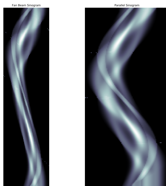
Figure 2. Sinogram examples: the new spectral phantom projection data at a projection interval of 1 degree. On the left, the projection data before resorting; on the right, the parallel projection data obtained after resorting the fan-beam line integrals.
