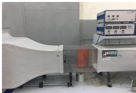
Figure 3. GUNT HM 170 wind tunnel and airfoil model mounted in the test section.
