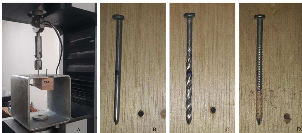
Figure 3. (A) Equipment setup used for the nail withdrawal tests. Typical failure modes: (B) Smooth-shank nails cause minimal damage to the wood; (C) Helical nails withdraw small amounts of wood fibers; (D) Annular nails extract a column of wood fiber fragments adhered to its threads.
