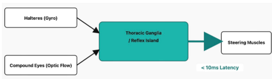
Figure 1. A schematic diagram illustrating the tight sensor-compute-actuation loop in Drosophila [1–5].
