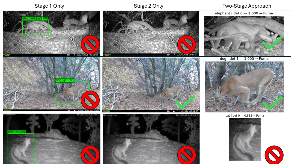
Figure 3. Illustrative examples comparing Stage 1-only, Stage 2-only, and the proposed two-stage pipeline. Columns report Stage 1 detector outputs, Stage 2 full-frame classifier outputs, and the two-stage decision (Stage 1 crop + Stage 2). Rows include two puma cases (nighttime partially occluded; daytime) and one non-target fox example that produces a puma-like false positive across methods (see Section 5.3).
