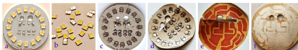
Figure 7. (a) LED module (E27-C), (b) SMD LEDs, (c) bare LED module, (d) top view of the detached PCB, (e) the rear view of the detached PCB with the electrical circuit and the insulating thin-film coating, (f) the aluminium substrate of the LED module (Authors' images).
