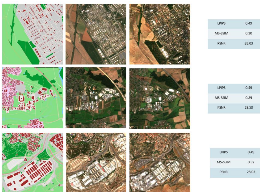
Figure 17. Samples of generated patches in TCI band from 1st test set (masks, real images, synthetic images) and associated quality measure values.
