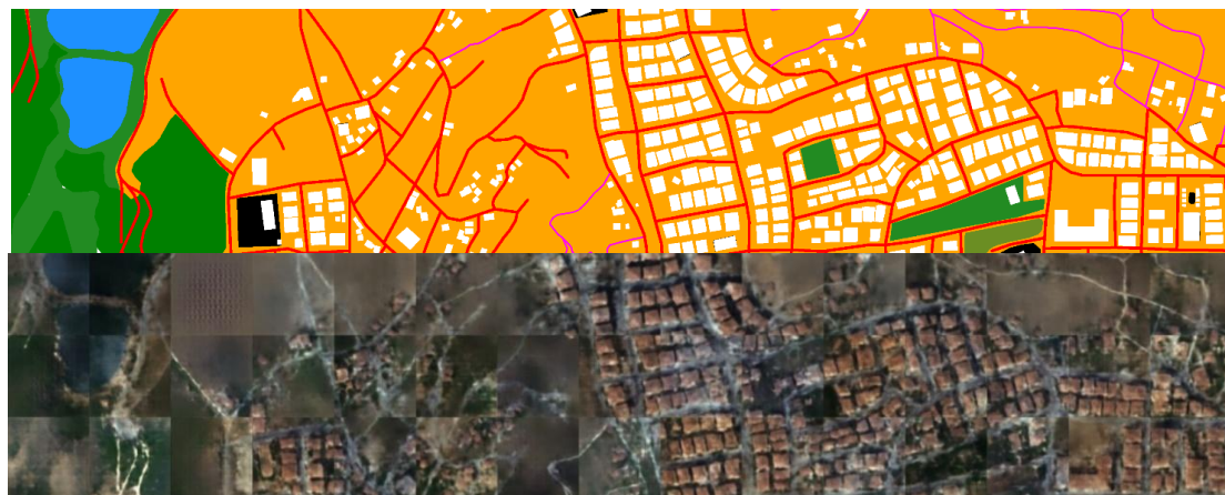
Figure 29. The map raster produced with the SkySat base (top) and the corresponding synthetic image generated (below).
