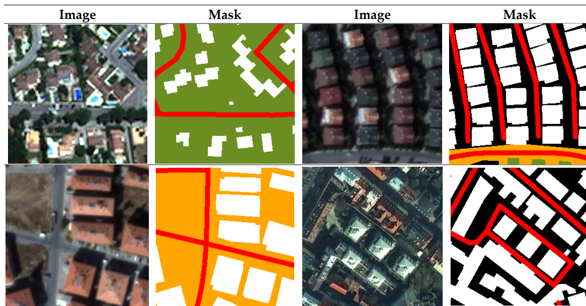
Figure 12. Images and corresponding masks from the Salon-de-Provence dataset (top left), Ankara dataset (top right and bottom left), and Munich dataset (bottom right).
