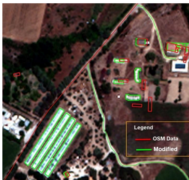
Figure 13. An example to the inconsistencies between the OSM data (red polygons) and the images. The corrected data is shown with green polygons.
