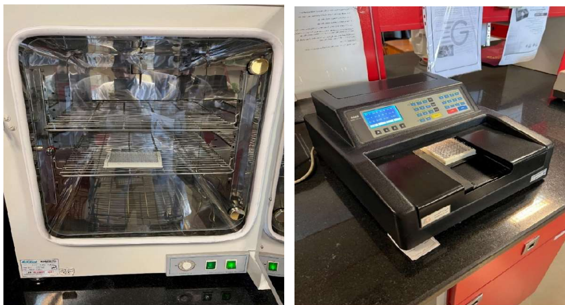
Figure 2. Equipment used in the experimental section, including incubator (left) and ELISA reader (right).
