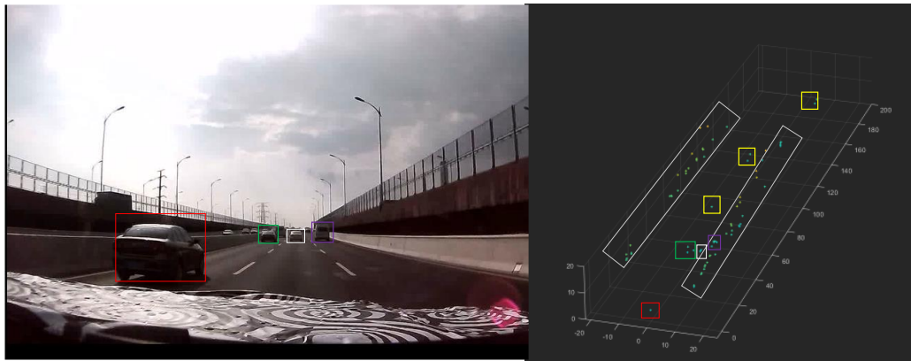
Figure 14. The display effect of vehicles during road testing, with nearby vehicles indicated by red, green, white, and purple boxes, and more distant vehicles marked with yellow boxes. the gray area represents the fence on both sides.
