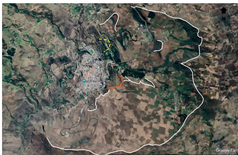
Figure 3. Aerial view of the Alausí landslide area (village at the center of the picture and the crown in dashed yellow line) showing several scarps (white lines) related to possible ancient mass movements, including the Cerro Gampala landslide scarp (in red line). Modified from Google Earth [17].
