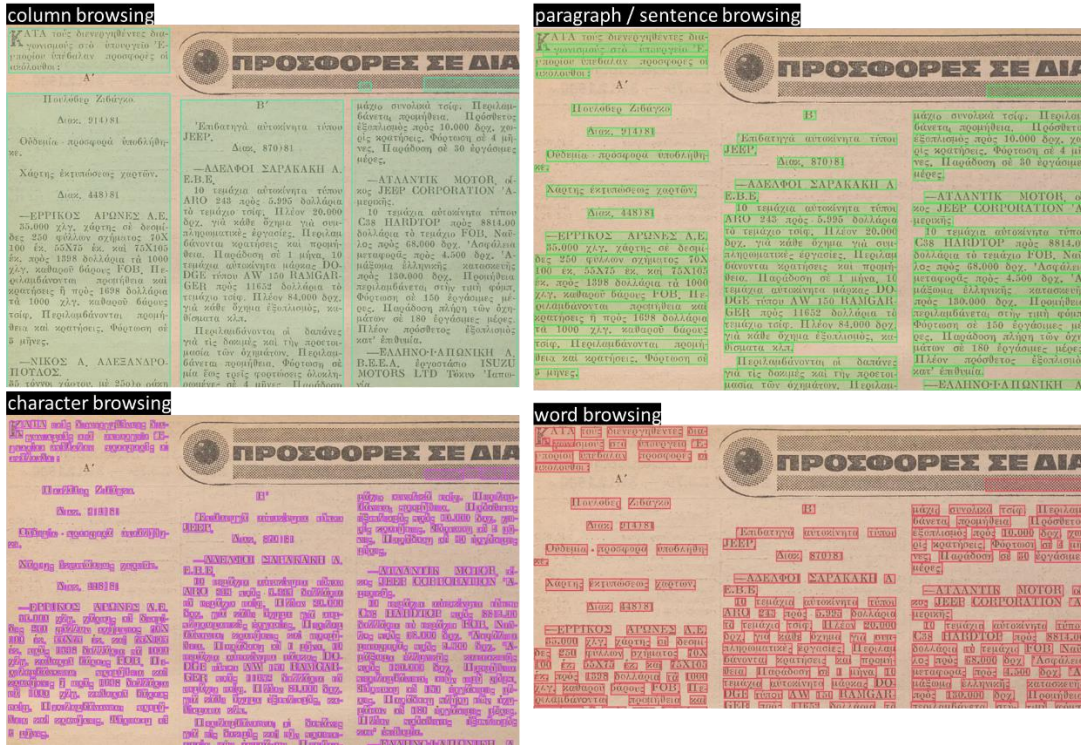
Figure 10. Exploiting the output metadata of OCR tools to provide information on recognized text regarding bounding rectangles at the level of columns, paragraphs, sentences, words and individual characters.
