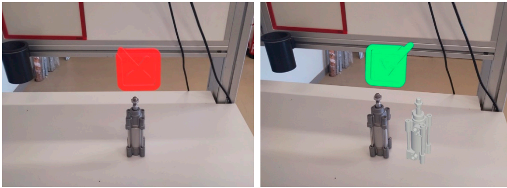
Figure 5. Validation process of the pneumatic cylinder assembly quality control.
