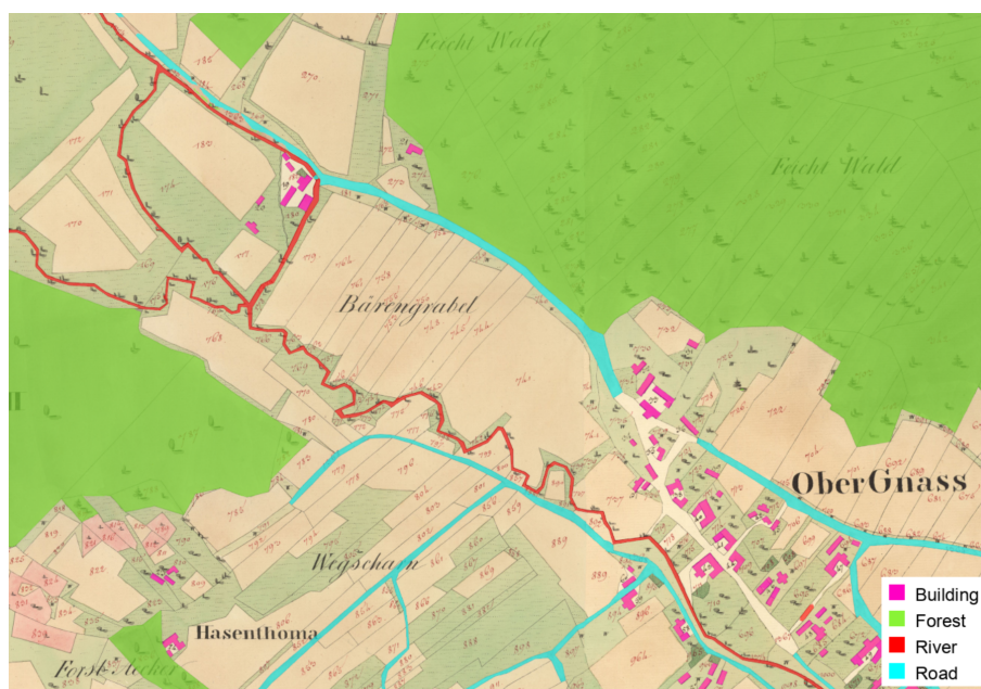
Figure 2. Georeferenced scan of a sheet of the Franziszeische Kataster after automatic segmentation.
