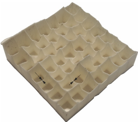
Figure 8. Location of measuring points for calculation of minimal thickness that can be successfully injection molded.
